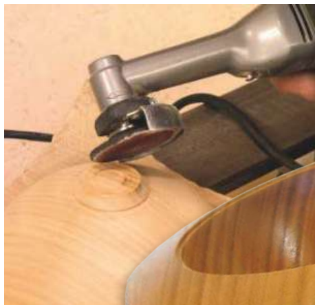
▲ Pic.32 You may find power sanding the interior difficult. I used a cordless drill for safety and this 3 o'clock position kept everything out of the way. Sand the edge with a block with the lathe switched off
